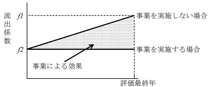
$$B_{a-2} \text{ (円)} = \sum_{t=1}^Y \frac{t \times (f_1 - f_2) \times \alpha \times A \times U}{Y \times 360 \times (1 + i)^t}$$
