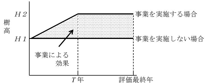
$$B_m \text{ (円)} = \left[ \sum_{t=1}^{T-1} \frac{t}{T \times (1+i)^t} + \sum_{t=T}^Y \frac{1}{(1+i)^t} \right] \times (H_2 - H_1) \times L \times U$$
