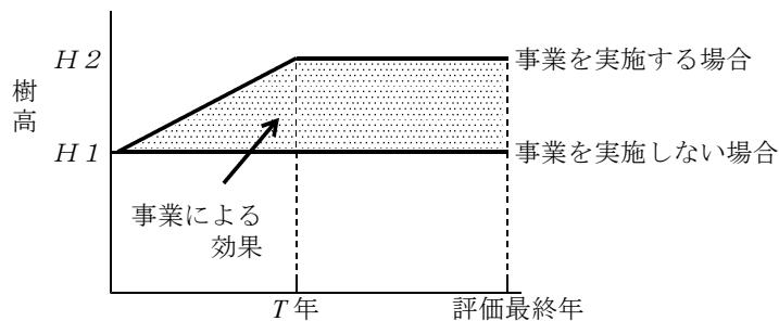
$$B_j \text{ (円)} = \left( \sum_{t=1}^{T-1} \frac{t}{T \times (1+i)^t} + \sum_{t=T}^Y \frac{1}{(1+i)^t} \right) \times (H_2 - H_1) \times L \times U$$
