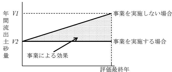
$$B_{d-2} \text{ (円)} = \sum_{t=1}^Y \frac{(V_1 - V_2) \times t \times A \times U}{Y \times (1 + i)^t}$$
