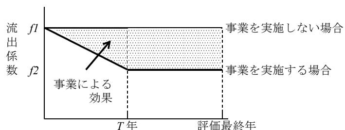
$$B_{a-1} (\text{円}) = \left( \sum_{t=1}^{T-1} \frac{t}{T \times (1+i)^t} + \sum_{t=T}^Y \frac{1}{(1+i)^t} \right) \times \frac{(f_1 - f_2) \times \alpha \times A \times U}{360}$$
