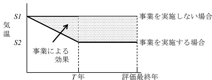
$$B_g \text{ (円)} = \left[ \sum_{t=1}^{T-1} \frac{t}{T \times (1+i)^t} + \sum_{t=T}^Y \frac{1}{(1+i)^t} \right] \times (S_1 - S_2) \times N \times D \times U$$
