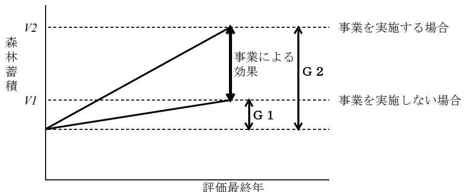
$$B_f \text{ (円)} = \sum_{t=1}^Y \frac{G2 - G1}{Y \times (1+i)^t} \times D \times BEF \times (1+R) \times 0.5 \times \frac{44}{12} \times U$$
