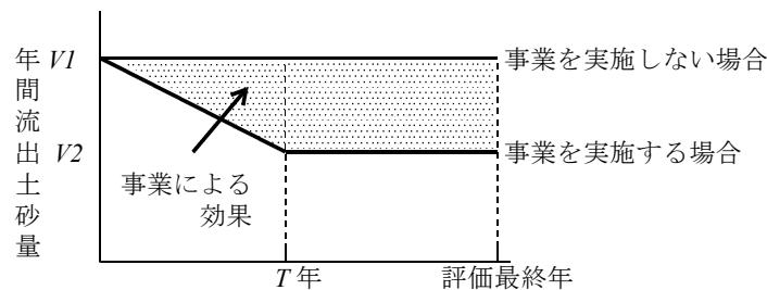
$$B_{d-1} \text{ (円)} = \left( \sum_{t=1}^{T-1} \frac{t}{T \times (1+i)^t} + \sum_{t=T}^Y \frac{1}{(1+i)^t} \right) \times (V_1 - V_2) \times A \times U$$
