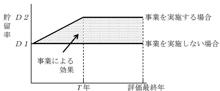
$$B_{b-1} \text{ (円)} = \left( \sum_{t=1}^{T-1} \frac{t}{T \times (1+i)^t} + \sum_{t=T}^Y \frac{1}{(1+i)^t} \right) \times \frac{(D_2 - D_1) \times A \times P \times U \times 10}{365 \times 86,400}$$
