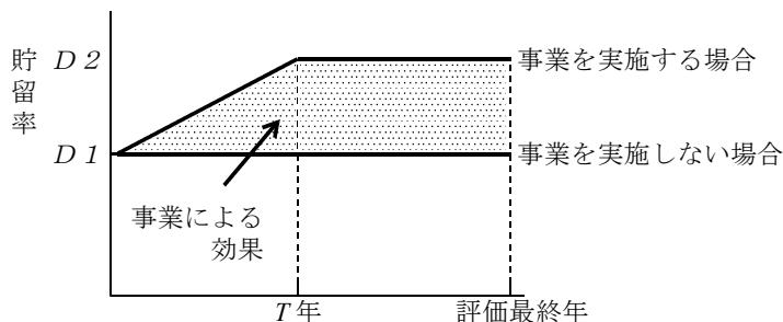
$$B_{c-1} \text{ (円)} = \left( \sum_{t=1}^{T-1} \frac{t}{T \times (1+i)^t} + \sum_{t=T}^Y \frac{1}{(1+i)^t} \right) \times (D_2 - D_1) \times A \times P \times u \times 10$$
