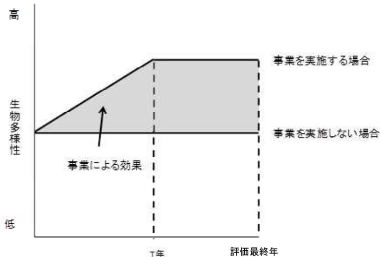
$$B \text{ (円)} = \left( \sum_{t=1}^{T-1} \frac{t}{T \times (1+i)^t} + \sum_{t=T}^Y \frac{1}{(1+i)^t} \right) \times D \times A$$
