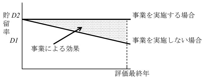
$$B_{b-2} \text{ (円)} = \sum_{t=1}^Y \frac{t \times (D_2 - D_1) \times A \times P \times U \times 10}{365 \times 86,400 \times Y \times (1 + i)^t}$$
