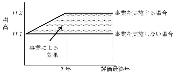
$$B_h \text{ (円)} = \left[ \sum_{t=1}^{T-1} \frac{t}{T \times (1+i)^t} + \sum_{t=T}^Y \frac{1}{(1+i)^t} \right] \times (H_2 - H_1) \times L \times U$$
