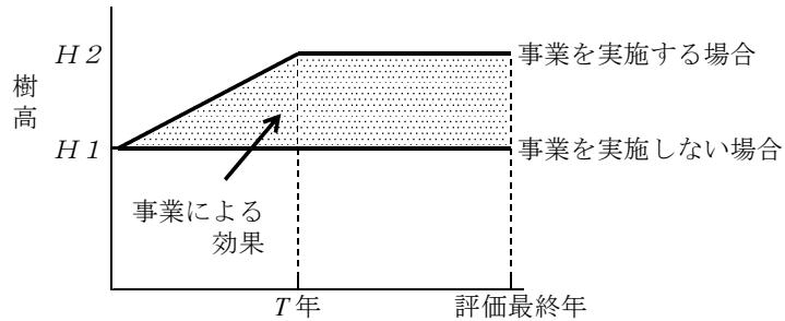
$$B_1 \text{ (円)} = \left[ \sum_{t=1}^{T-1} \frac{t}{T \times (1+i)^t} + \sum_{t=T}^Y \frac{1}{(1+i)^t} \right] \times (H_2 - H_1) \times L \times U$$
