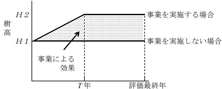
$$B_i \text{ (円)} = \left( \sum_{t=1}^{T-1} \frac{t}{T \times (1+i)^t} + \sum_{t=T}^Y \frac{1}{(1+i)^t} \right) \times (H_2 - H_1) \times L \times U$$
