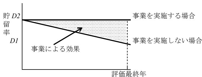
$$B_{c-2} \text{ (円)} = \sum_{t=1}^Y \frac{t \times (D_2 - D_1) \times A \times P \times u \times 10}{Y \times (1 + i)^t}$$
