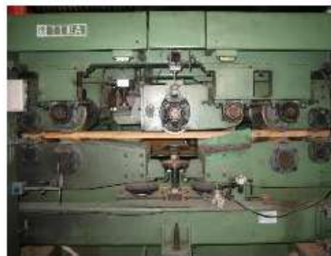
Figure 4-3: Inside a Continuous Grading Machine Photo: Saito Wood Industry Co. Ltd.
