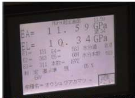
Figure 4-2: Recording the Calculated Young's Modulus of the Lamina into the Computer Photo: First Wood Co., Ltd.
