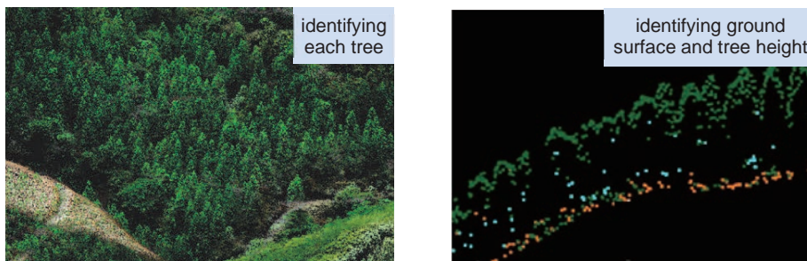
Fig. 8 Aeronautical laser measurement results
