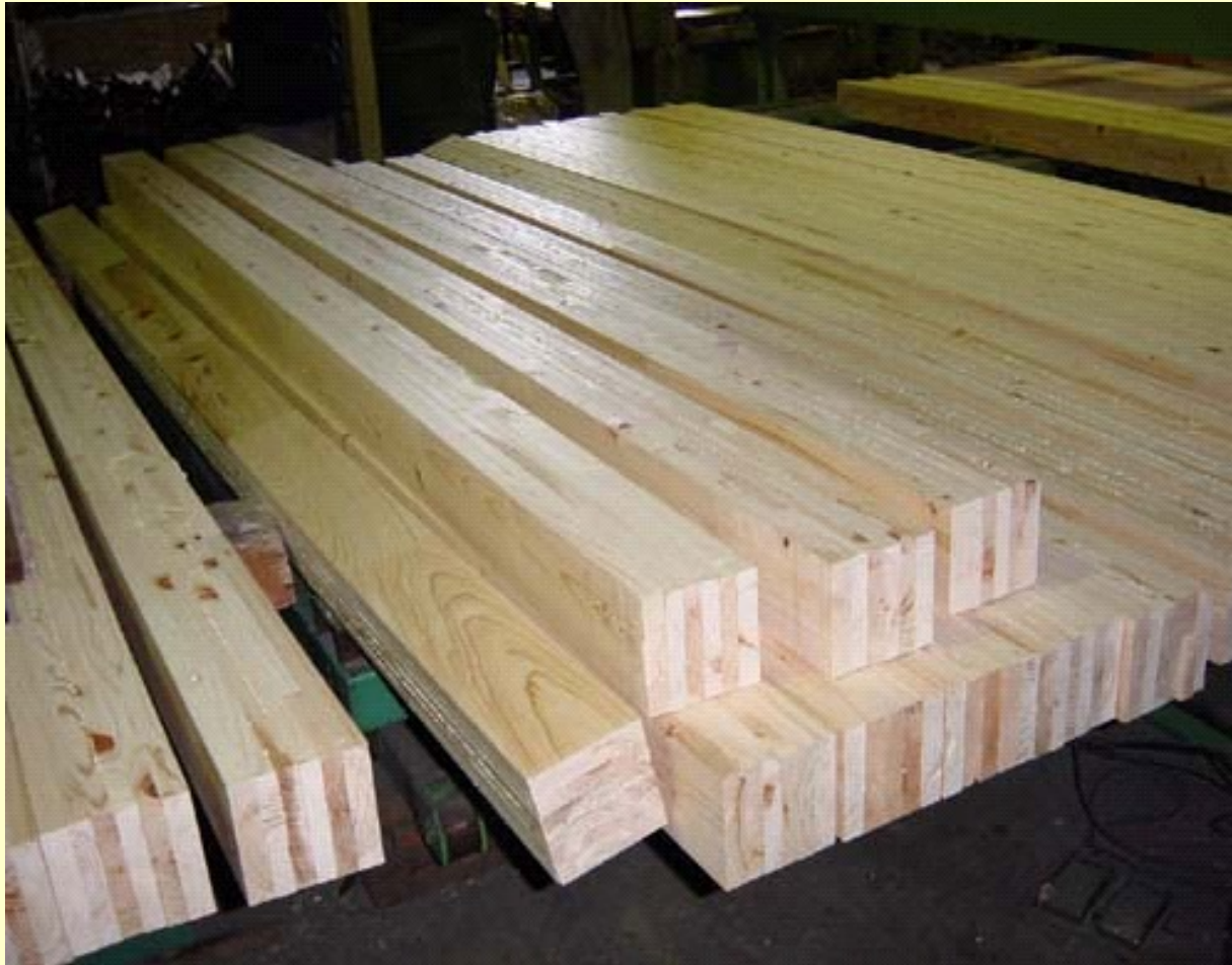
Engineered wood for use as poles (Japanese cypress)
