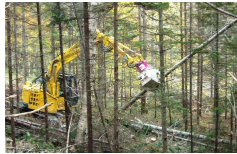
Row-thinning using high-performance forestry machinery (National forest in Ashoro) [Tokachi Tobu District Forest Office]
