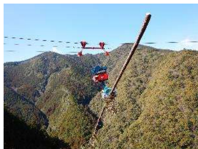
Remote-controlled skyline logging cable winche
