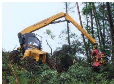
Advanced forestry machinery capable of logging to timber processing (Harvester)
