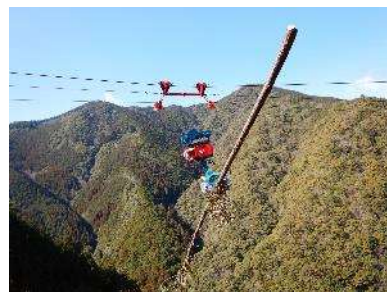
Remote-controlled skyline logging cable winche
