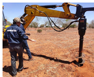
Excavation of planting holes using construction machinery
