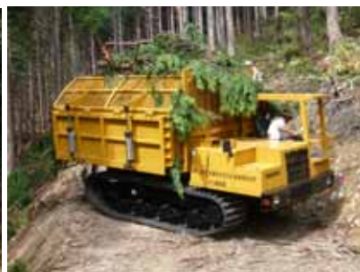
Forwarder for logging residue collection
